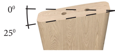
2. Cut the top of the leg into the desired angle
